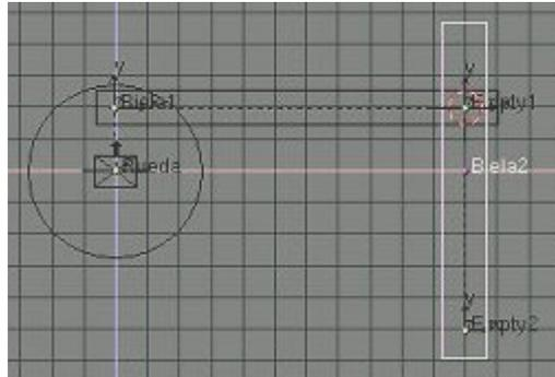
The idea is that both crankshafts will be joined together using this points (Empty1 and Empty2) like an articulation.
